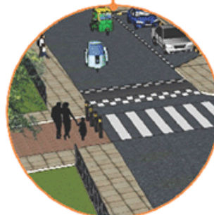
Segregated and connected NMT routes
